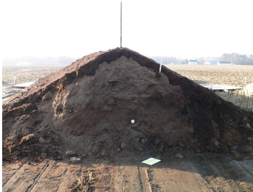
Picture 3. This illustrates how the wet layer forms on top of the pile and along the edges of the pile. This image was taken on 2 Feb 2006 from a pile that was created on 1 Nov 2005; this pile had received 9.8 inches of rain since 1 Nov 2005.
