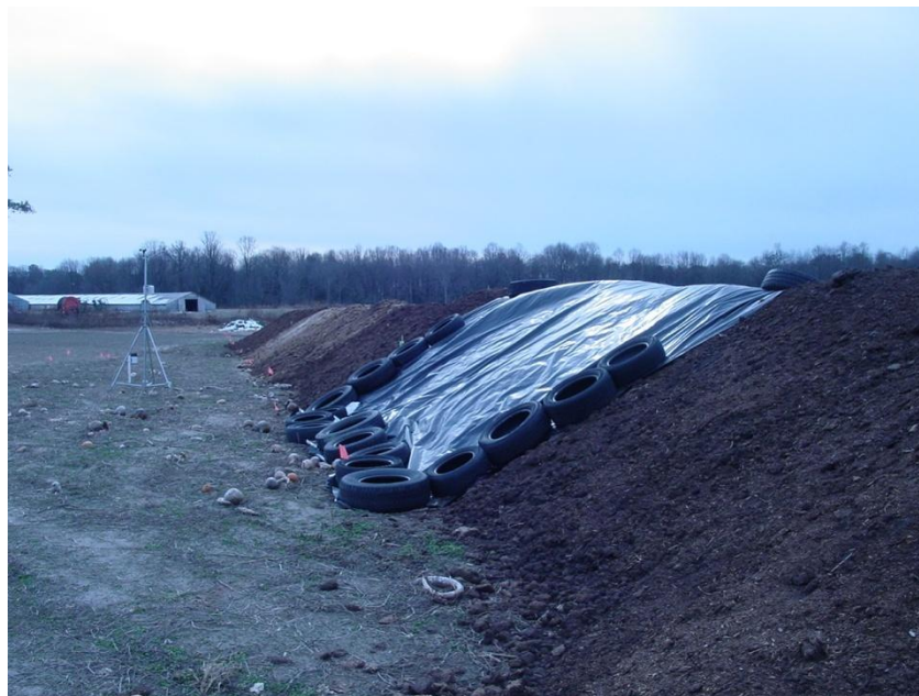
Picture 1. Site CB showing the no-cover treatment in the front, then the poly cover, then the bentonite base, then the two spray-on carbon treatments, then the sawdust treatment, and the Poultry Guard®-base treatment at the far end of the pile.
