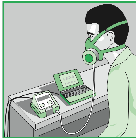
In a quantitative fit test, a particle-counting instrument is used to measure respirator fit.
