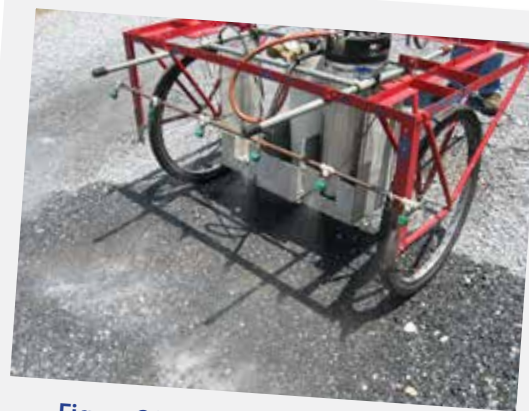
Figure 20. Evaluating nozzle and tip performance before calibration
