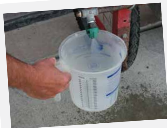
Figure 23. Capturing nozzle discharge
