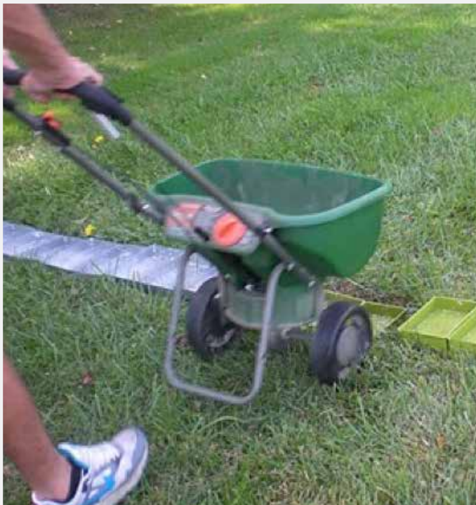
Figure 11. Fertilizer catch pans placed at regular intervals
