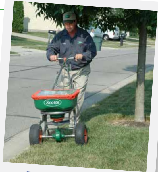
Figure 16. A deflector shield is used along a curb
