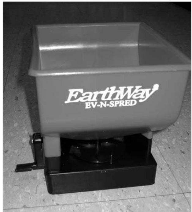
A broadcast spreader, one of several methods for applying pellet or granular herbicides, can be used on land or fitted onto a boat.
