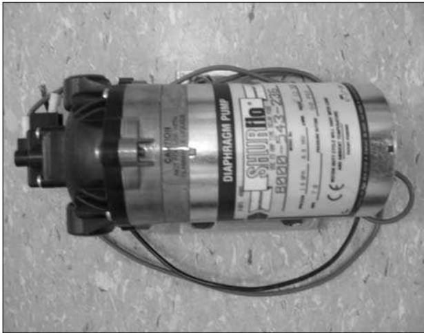
A diaphragm pump is an economical way to spray corrosive or abrasive herbicides, especially where units are driven by gas or diesel engines.
