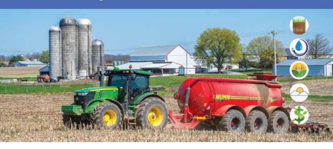
This practice uses special equipment to incorporate manure into the soil instead of spreading it on the surface.
