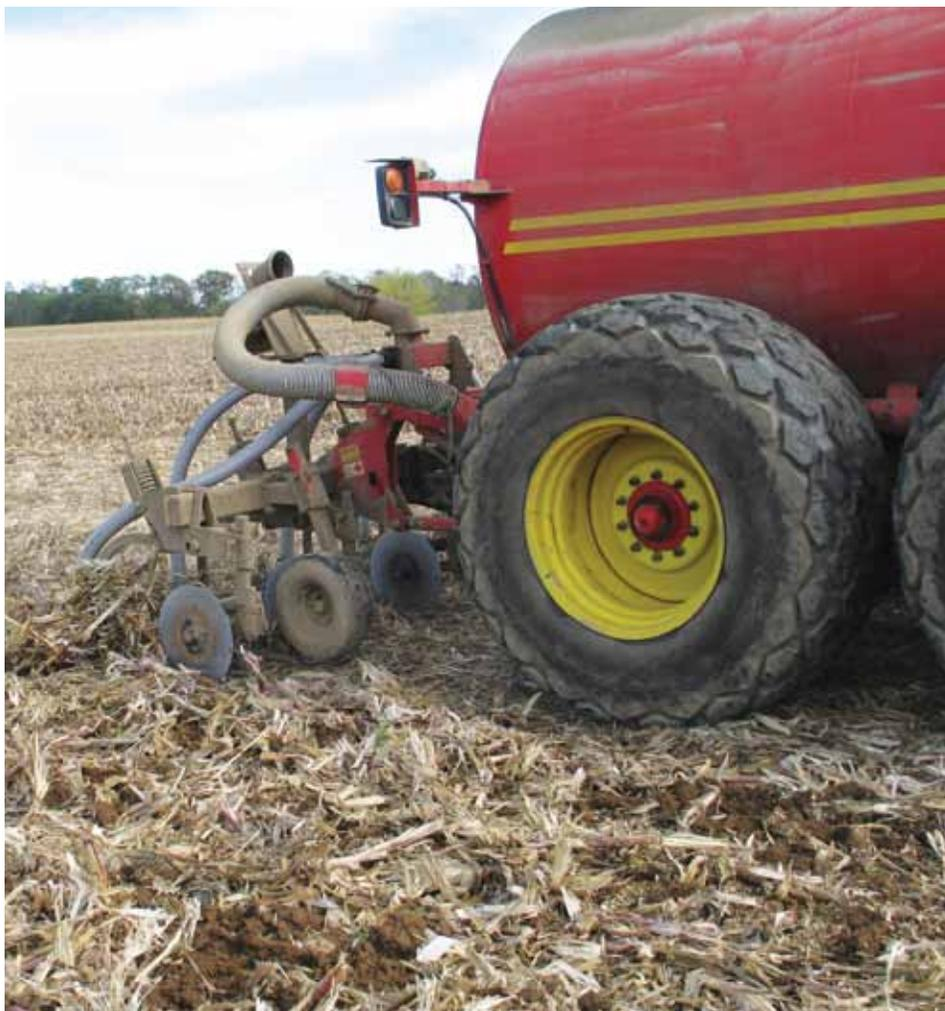
MANURE INJECTION AND INCORPORATION HELPS PREVENT NITROGEN AND PHOSPHORUS FROM IMPACTING WATERWAYS AND REDUCES ODORS.
