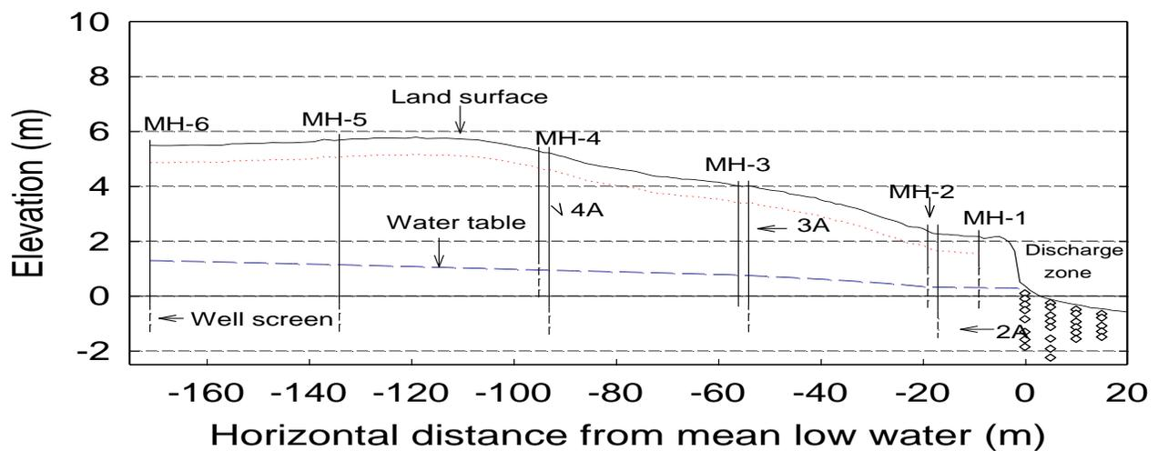
Figure 2. Cross-section of the study area and the monitoring system used to track the effects of cover crop use on nitrate-nitrogen delivered to the Wye River.
