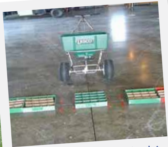
Figure 12. Fertilizer catch pans placed at regular intervals
