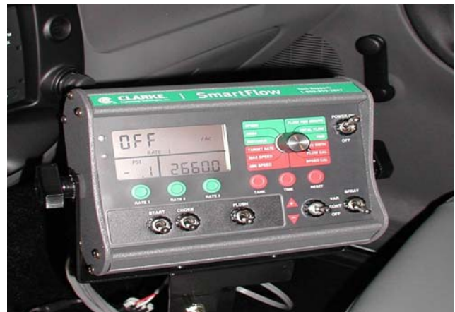
Figure 6.9 B. Truck cab mounted flowmeter for ULV sprayer.
