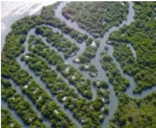
Figure 6.3. Open marsh water management (OMWM) creates a system of ditches and ponds that create additional aquatic habitat, increase fish populations and increase the frequency of tidal inundation, all of which help in the control of mosquitoes.
