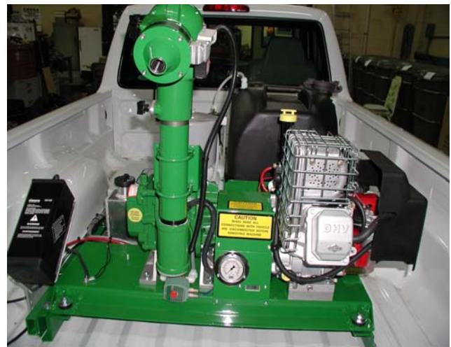
Figure 6.9 A. Truck mounted ULV sprayer.
