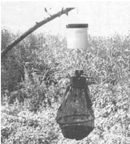
Figure 5.5. Battery operated CDC miniature light trap.
